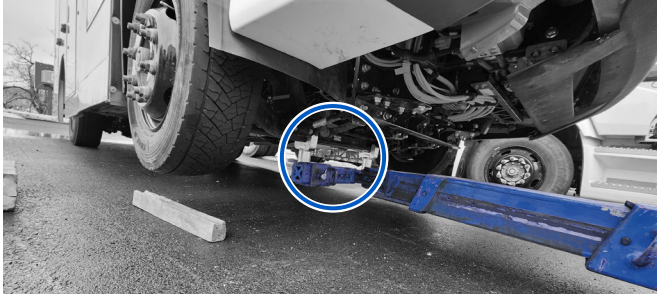
Figure 37 - Raising the front axle
