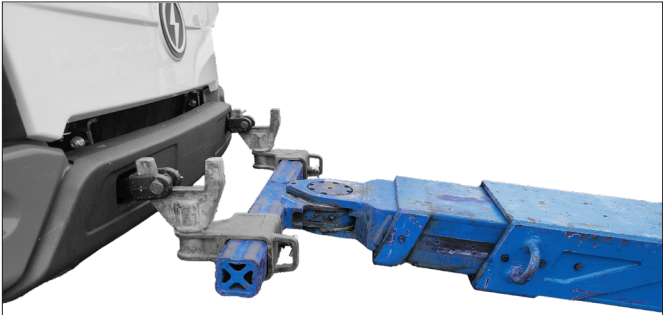
Figure 36 - Lifting by the front hooks
