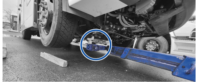
Figure 37 - Raising the front axle
