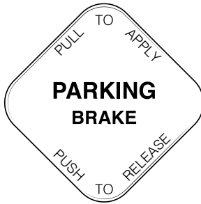
Figure 4 - Parking brake knob (yellow)
