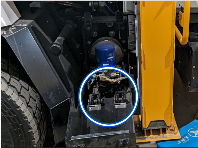
Figure 21 - Tow hooks, dowel pins and spring pins
