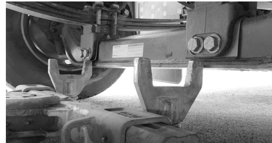
Figure 28 - Towing adapters and front axle
