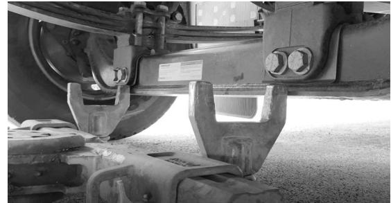
Figure 28 - Towing adapters and front axle
