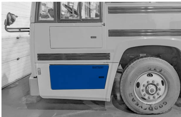
Figure 24 - 12 V battery compartment
