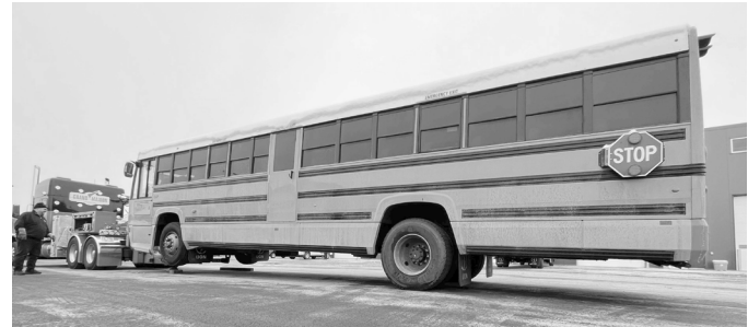
Figure 38 - Lion D lifted by the front axle
