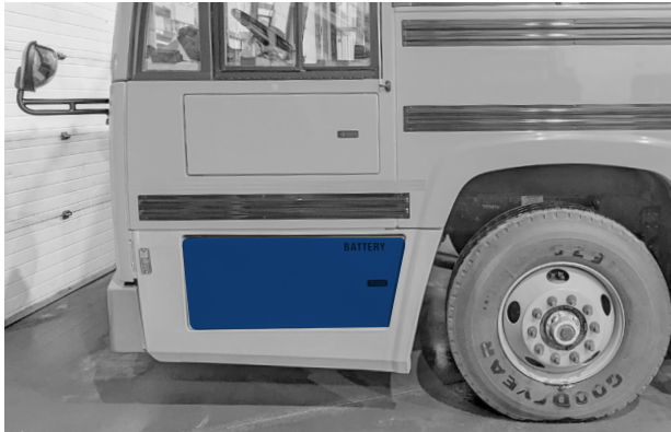
Figure 24 - 12 V battery compartment
