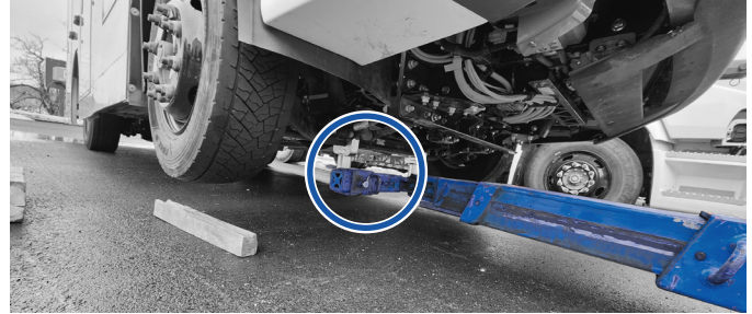
Figure 12 - Raising the front axle
