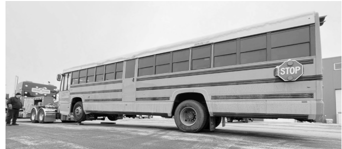
Figure 5 - Lion D lifted by the front axle
