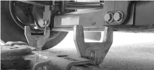
Figure 4 - Tow truck's crossbar and lift adapters
