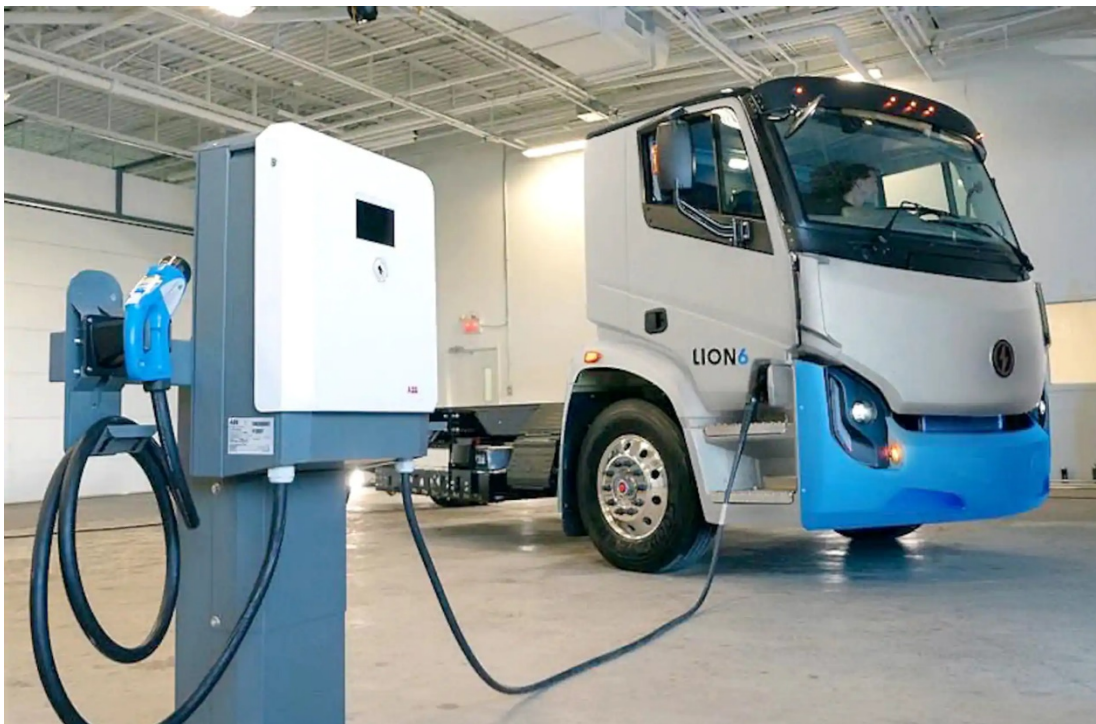
Lion6 all-electric truck and Terra DC Wallbox ABB terminal
