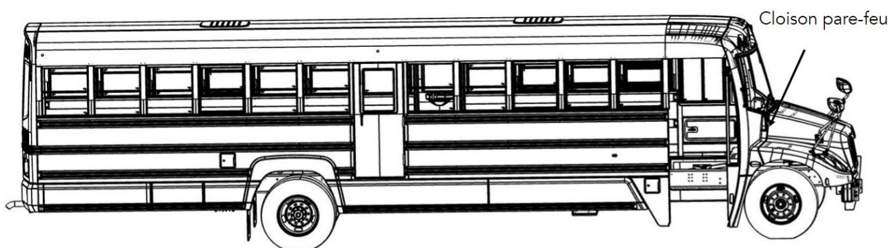
Figure 1 - Emplacement de la cloison pare-feu
